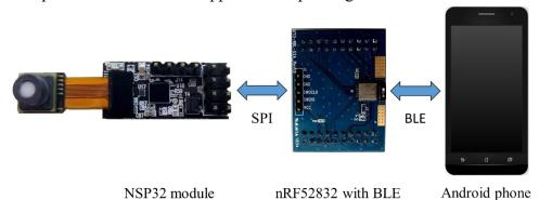
A Nordic nRF52832 SoC acts as a forwarder, to forward command packets and return packets between the NSP32 module and the Android phone, where the Android app can wirelessly (through bluetooth) control NSP32 module and get the spectrum data.
