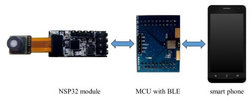
Note: Users can replace the BLE with WIFI or other wired/wireless transmission protocols.
